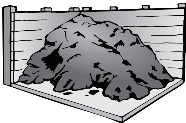
Example of mixing/storage area with buck wall.
