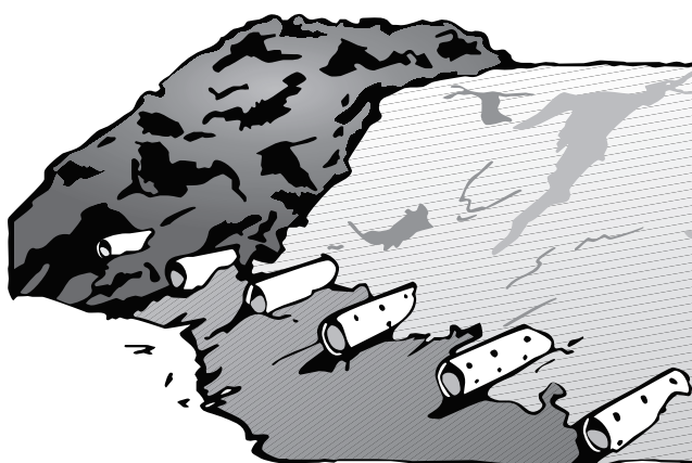
Aerated static pile with perforated PVC pipes.
