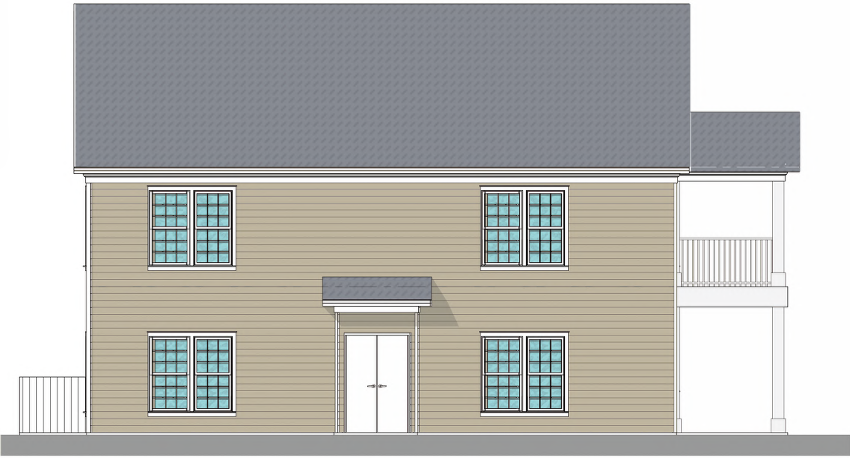
1 APARTMENT ADDITION - NORTH ELEVATION A-201 1/4" = 1'-0"
