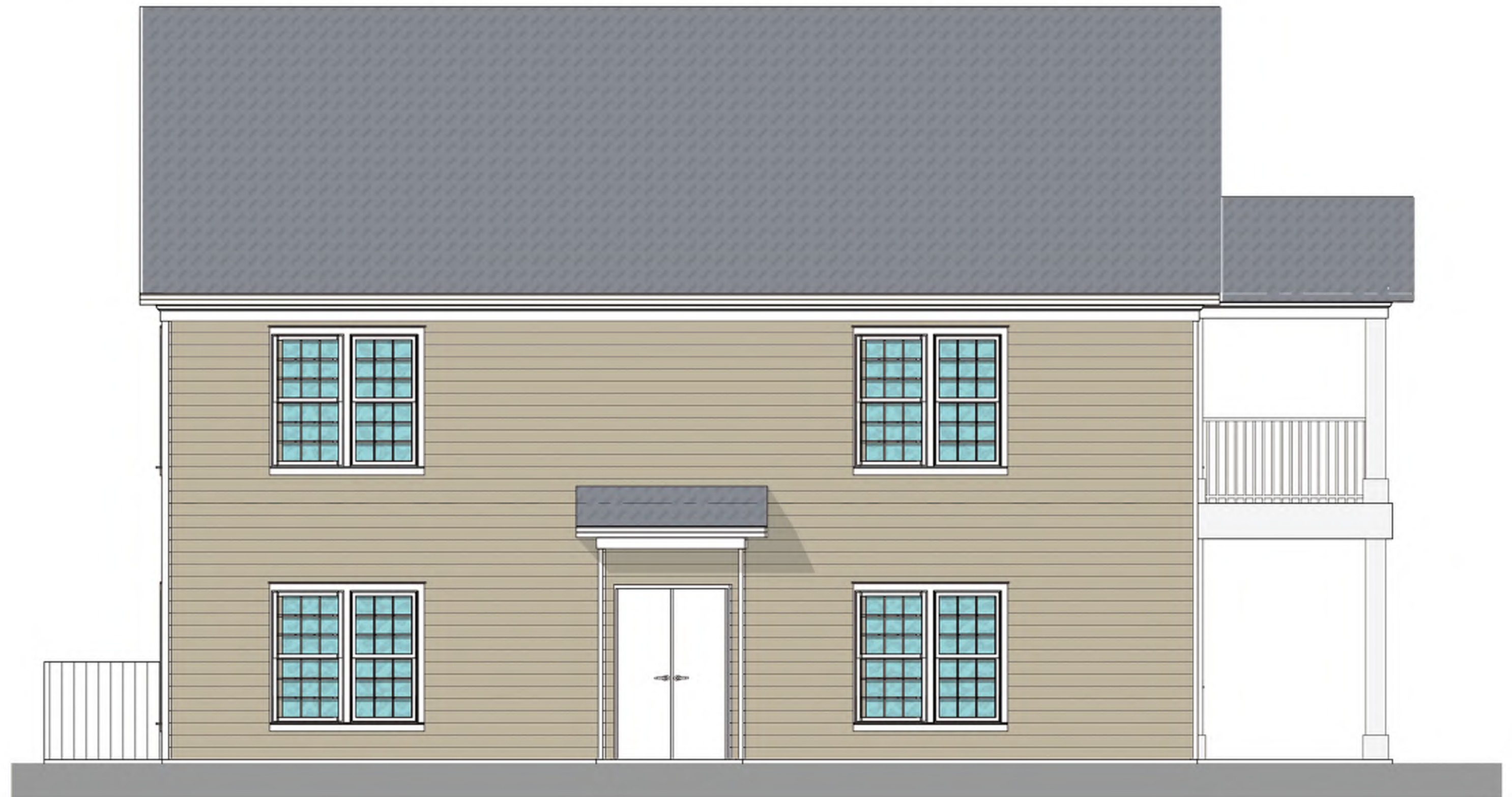
1 APARTMENT ADDITION - NORTH ELEVATION A-201 1/4" = 1'-0"
